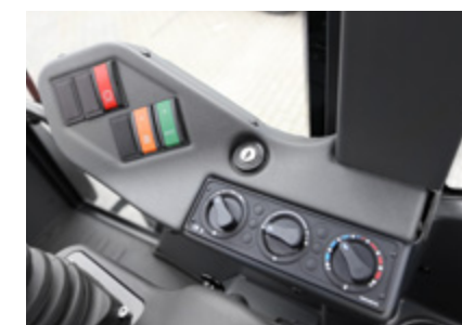
Ignition switch, controls for the heating and optional air-conditioning system are easy to reach
